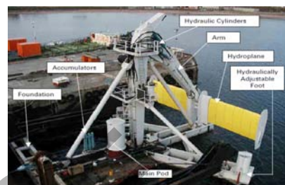
figure 4: Stingray Tidal Stream Generator
