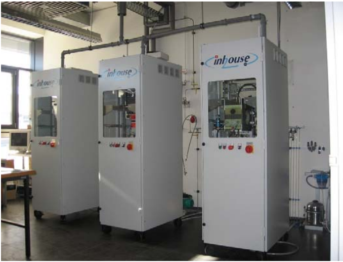
Figure 1. Fuel cell test benches "Reformate", "Hydrogen" and "Experimental" (from right).
