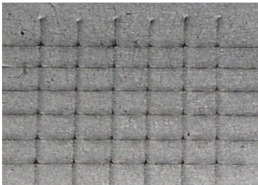
Figure8. View of the sample after cross-cut test
