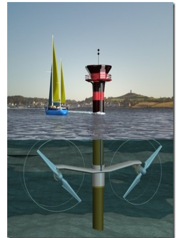
figure 3: Tidel turbines (horizontal-axis propeller design)
