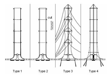
Fig. 3: different kinds of chimney construction
