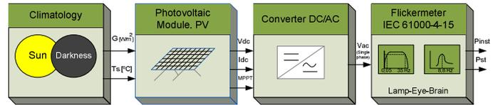
Figure. 1. Block diagram of the whole system.
