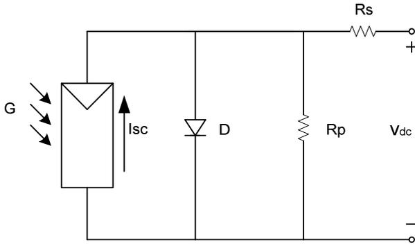
Figure. 2. Equivalent circuit model of a solar cell.
