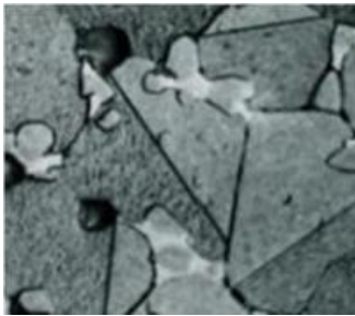
Figure 2. ZnO ceramic structure
