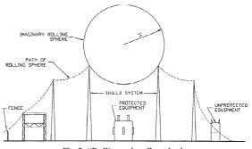
Fig.2. "Rolling sphere" method
