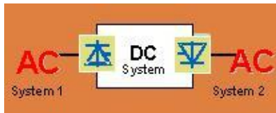
Fig 2. Simplification scheme of HVDC transmission
